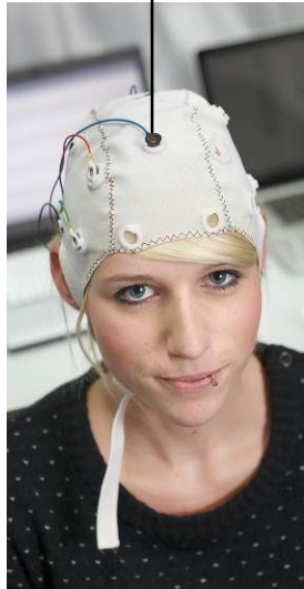
Figure 2 EEG cap with positions measured during the experiment. Nose points upwards. Picture of subject with corresponding electrode marked.
