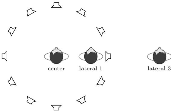
(b) The tested listening positions; *lateral position 1* is 1 m off-center, *lateral position 3* is 3 m off-center
