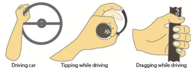
Figure 1 illustrates microgestures that would allow automotive control without releasing the steering wheel.
