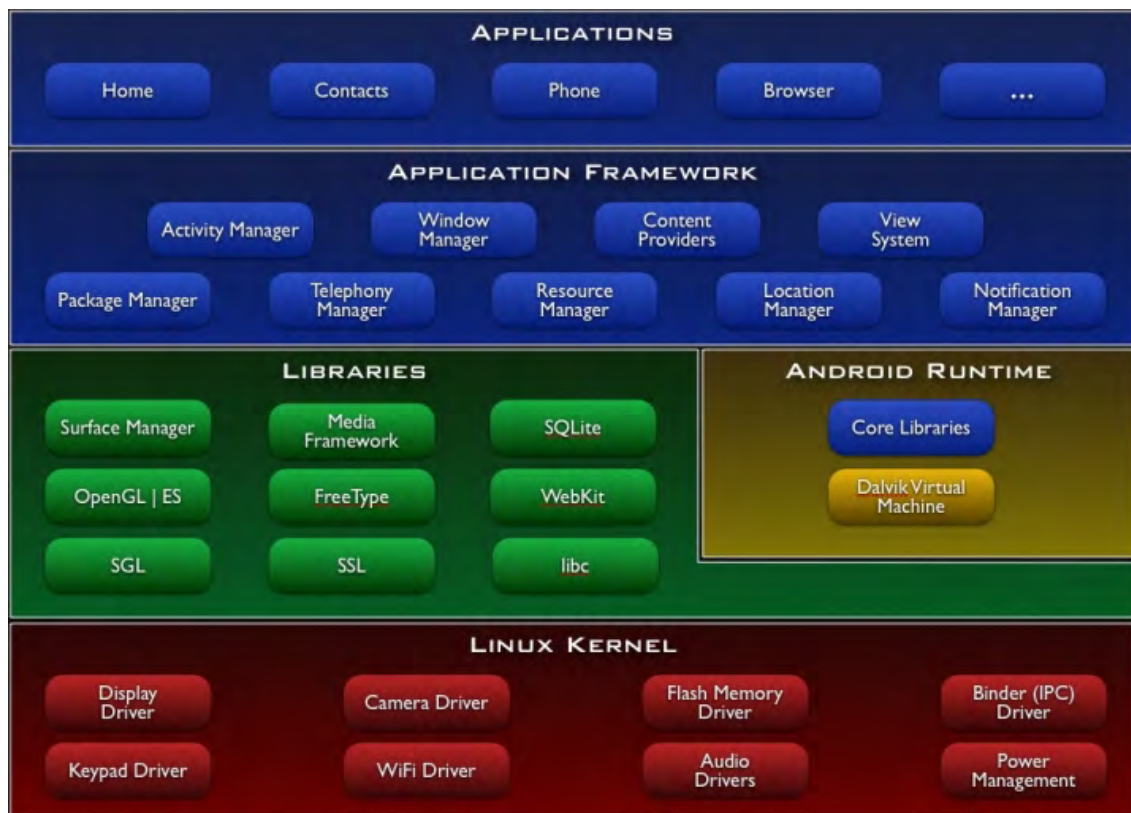
Figure 4.3: Architecture and components of the Android-System [61]
