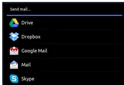
Figure 4.5: Screenshot of chooser with Apps for E-Mail Intents on Honeycomb HTC Flyer
