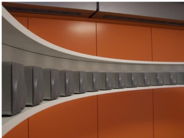
**Fig. 1:** A section of the loudspeaker array which was re-synthesized via headphones. The system is circular with a nominal radius of 1.495m and is composed of 56 equiangularly spaced loudspeakers.
