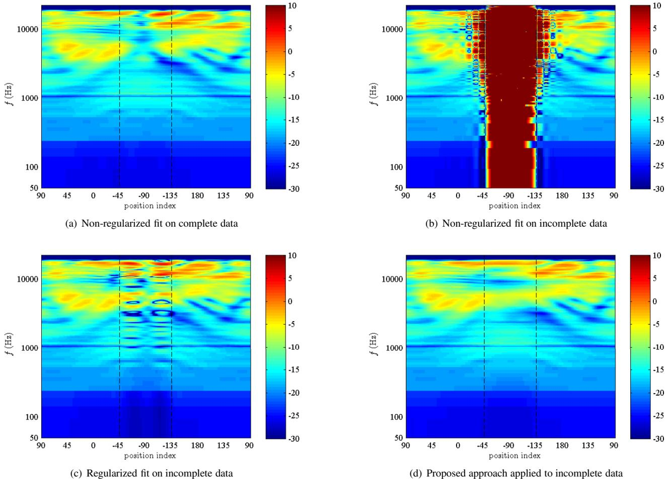
**Fig. 2.** HRTF magnitudes in dB along the great circle shown in Fig. 1(b) reconstructed from different types of least-squares fit. Position index 0 represents the corresponding direction in the frontal horizontal plane and positive indices represent the upper hemisphere, negative indices represent the lower hemisphere. The left half of the plot thus represents the frontal hemisphere; the right half represents the rear one. The area between the black vertical lines represents unknown data.
