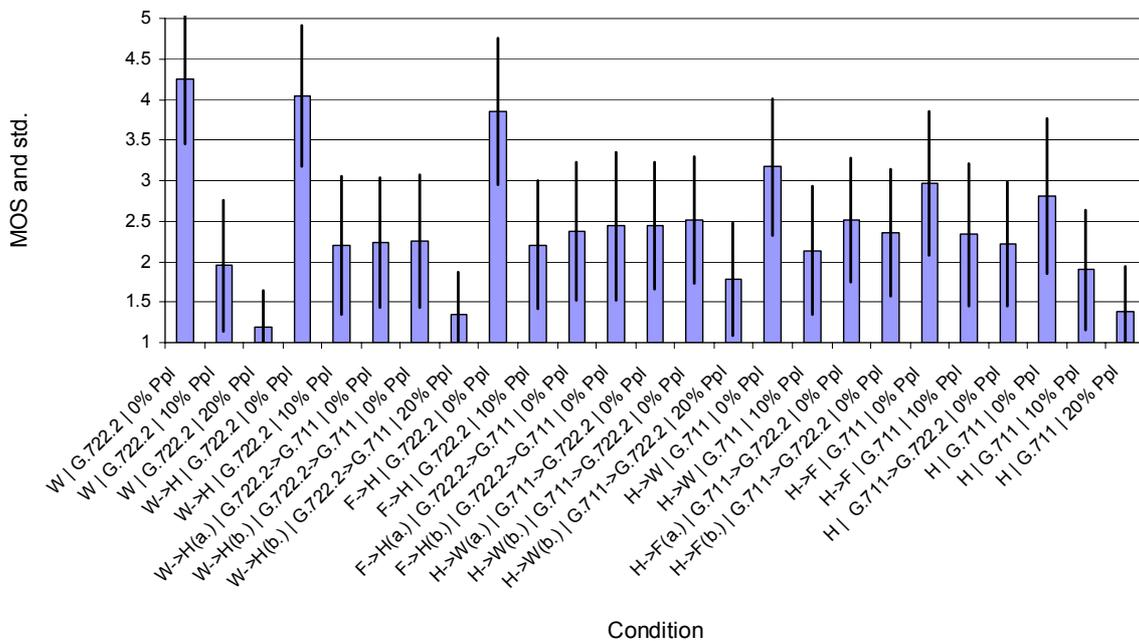
**Figure 2:** Results of Test 2a. First field: network conditions: W: WLAN; H: HSDPA; F: Flash-OFDM; →: network handover; (b.): codec changeover before network handover; (a.): codec changeover after network handover. Second field: codec conditions: G.711: G.711 at 64 kbit/s; G.722.2: G.722.2 at 23.05 kbit/s; →: codec changeover. Third field: packet loss conditions.
